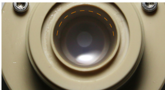
Figure 2: Top view of TSC spectro after spectroelectrochemical experiment using TMPD as analyte. The lower compartment, in which the working electrode is located, is blue coloured due to formation of the radical cation, while the upper part above the membrane (see the white bubble that formed under it for its exact location) is still transparent. The dotted orange line is displayed as guide for the eye to locate the upper filling level of the transparent part of the solution.
