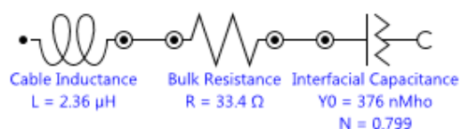
Figure 2a: Equivalent circuit representing the impedance behaviour of the KOH solution in contact with two platinum electrodes within the chosen frequency range.
