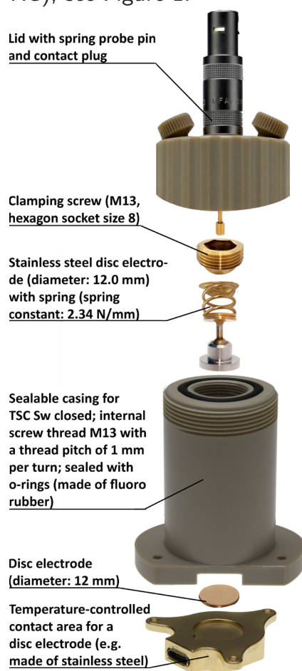
Figure 1: Exploded view of measuring cell TSC Sw closed for studies on solid and polymeric samples. To control the sample's temperature, the TSC Sw closed has to be used in combination with a Microcell HC setup.
