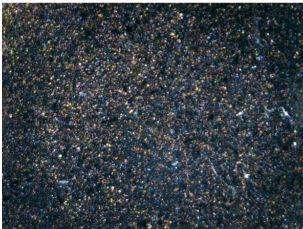
Figure 3. Micrographs of the graphite electrode during the various stages of lithiation. All micrographs have the same scale and show the same area of the electrode.
