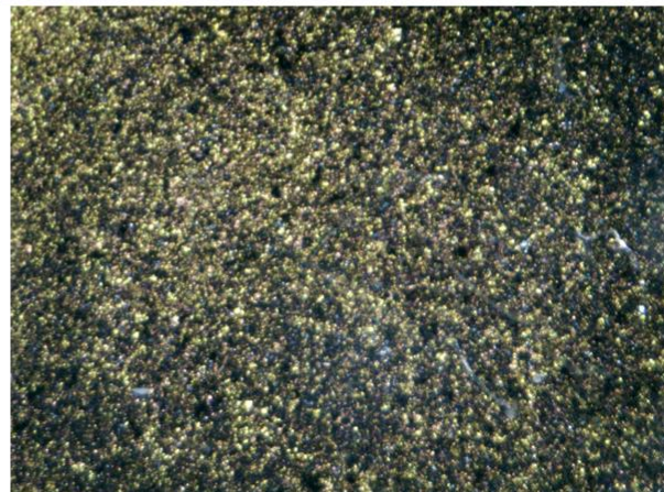
Figure 3. Micrographs of the graphite electrode during the various stages of lithiation. All micrographs have the same scale and show the same area of the electrode.
